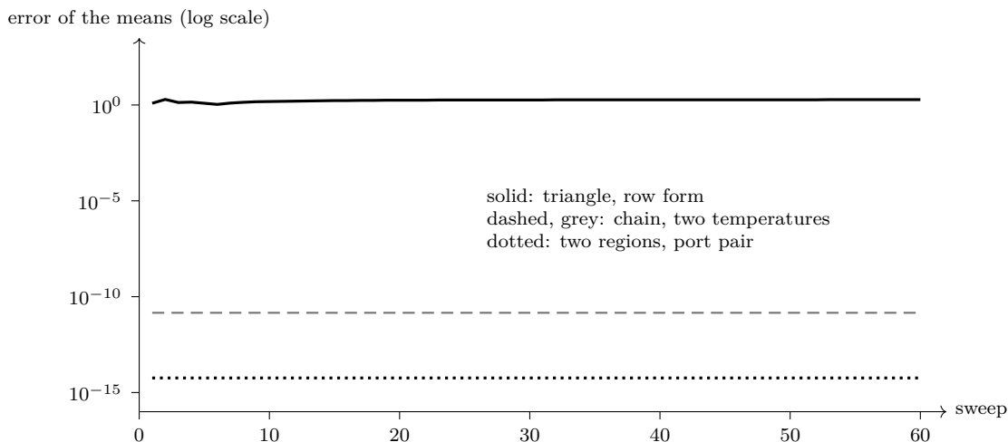
Figure 9.1: Gaussian belief propagation sweep by sweep: the largest error of the belief means against the exact posterior, on a logarithmic scale. Solid: the DC triangle in row form, radius 1.70; the error wanders between one and two, a hundred to two hundred percent, and never settles. Dashed: the chain reduced to its two temperatures, radius 0.20. Dotted: the two-region network reduced to its port pair, radius 0.29. Both reductions are trees and are exact after one sweep.
